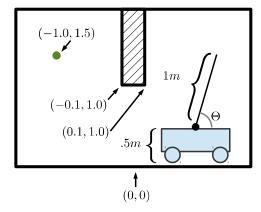
• Draw the configuration space for this robot, with x on the horizontal axis and  $\theta$  on the vertical axis. Draw  $C_{obs}$  as a shaded region. (6pts)
