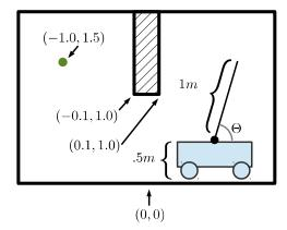
• Draw the configuration space for this robot, with x on the horizontal axis and  $\Theta$  on the vertical axis. Draw  $\mathcal{C}_{obs}$  as a shaded region. (6pts)
