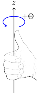
Figure 4: Right-hand rule for determining the direction of positive rotations around an axis.
