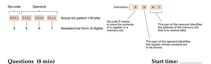
5. How many bits is the op-code? How many possible op-codes can the machine support?
