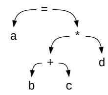
load b  $\rightarrow$  r1 load c  $\rightarrow$  r2 add r1, r2  $\rightarrow$  r3 load d  $\rightarrow$  r4 mult r3, r4  $\rightarrow$  r5 store r5  $\rightarrow$  a
