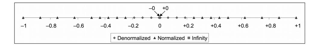
Representable values for 6-bit floating-point format. There are k = 3 exponent bits and n = 2 fraction bits. The bias is 3.
