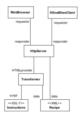
It illustrates, at a fairly high level, the important concepts in the system (note that the WWW browser is not part of the system). It is not intended as an engineering design. That is, the software components that need to be designed and developed may or may not correspond to these concepts.
